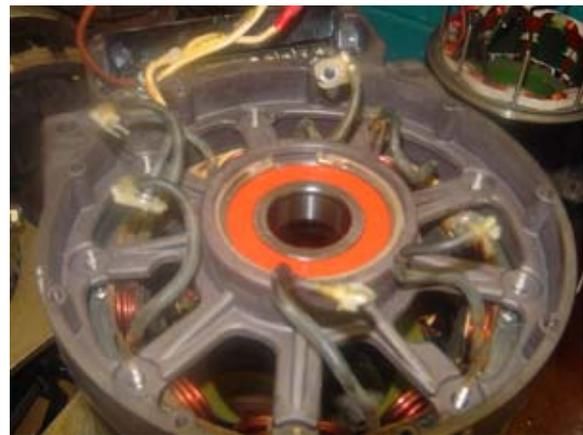
Figure 3—Phase Leads and Field Coil Leads
