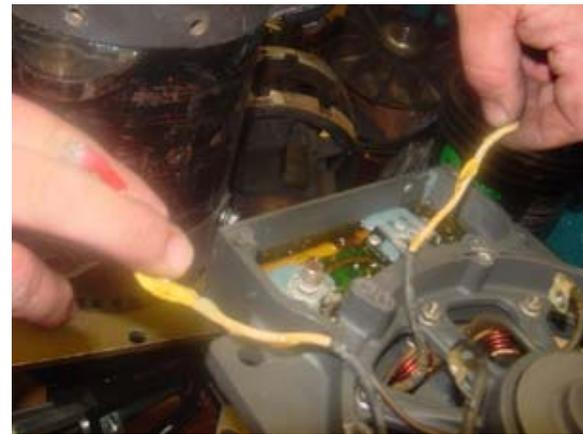
Figure 4—Field Coil Leads
