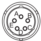
Figure 7 – Alternator-to-Regulator 5-Pin Harness Plug
