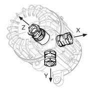
Figure 1: C192/C193 Gland Locations (unit is shipped with gland in one of three orientations)
