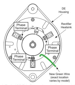
Figure 2: Typical DE Side Connections (varies by model)
